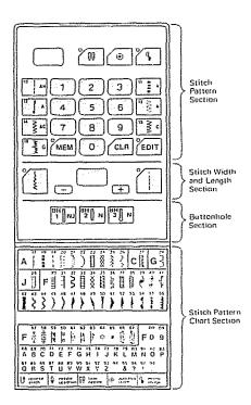
The Control Panel is divided into four sections:
